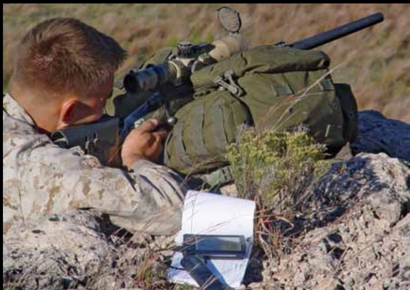
Here, a Marine is putting his ballistic PDA and Kestrel weather station to good use. With the effective use of these two tools, it is possible to have all of your rifle's data with any load you choose under any conditions with just a few minutes of work.
