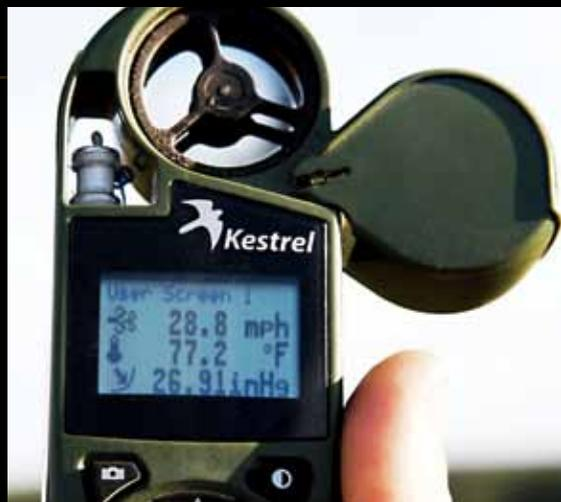
**The Kestrel portable weather station is crucial for effective measurement of weather conditions. Changes in pressure and temperature both significantly impact the trajectory of the bullet, so it is critical that we measure them accurately.**
