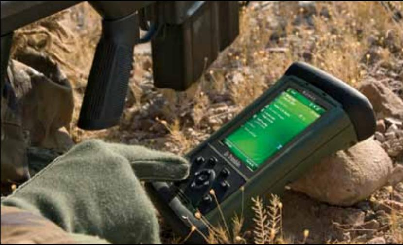
The ballistic solver works with any caliber, big or small. Once we enter in our weather conditions, muzzle velocity and ballistic coefficient, it's all science after that.
