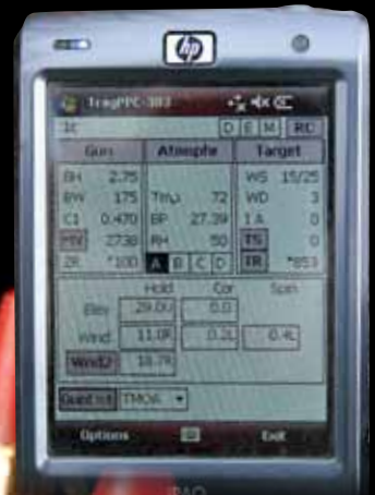
This is a typical screen shot of a ballistic solver. The three top tables represent our gun's information, atmospheric conditions and target distance and speed. The bottom tables give us our holds for both elevation and wind.
